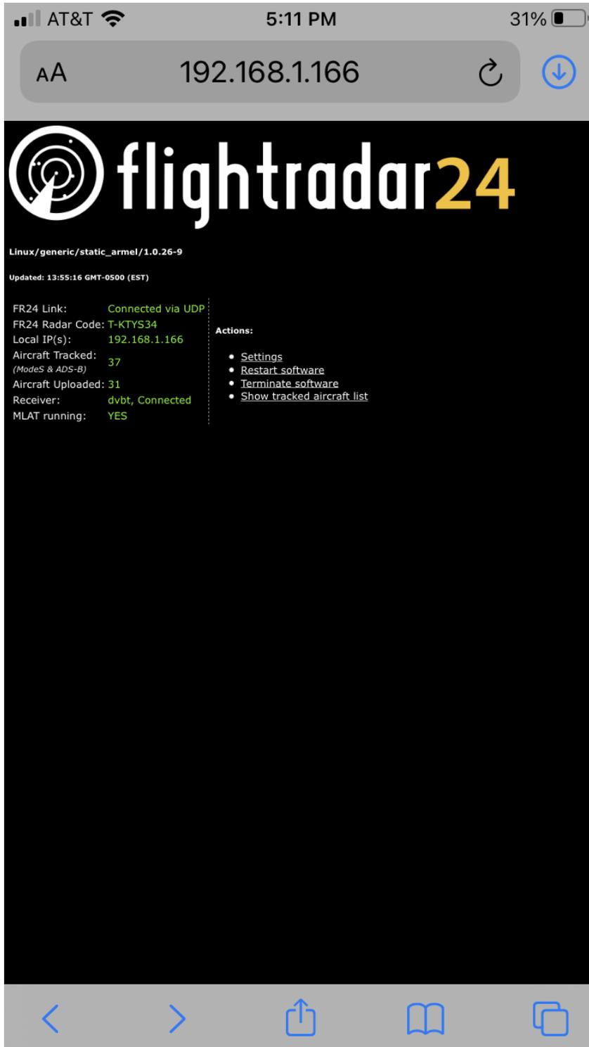
Flightradar24 display using the 4-Element Vertical Dipole Array. Aircraft detection range is approximately 100 miles.
